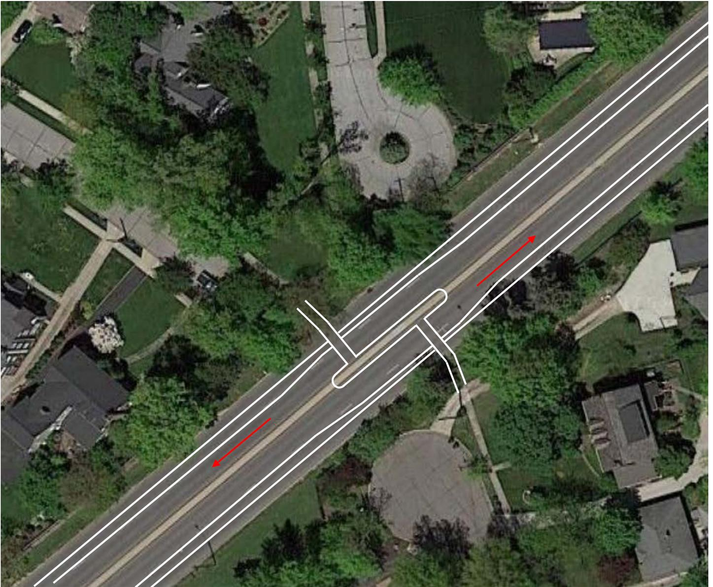
Two-stage crossing RRFB with a refuge island installed. This requires the narrowing of the bike buffer area to accommodate the median island.
